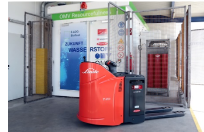
Austrian flagship project: demonstration of fuel-cell range extender warehouse trucks (JR: LCSA, monitoring tasks)
